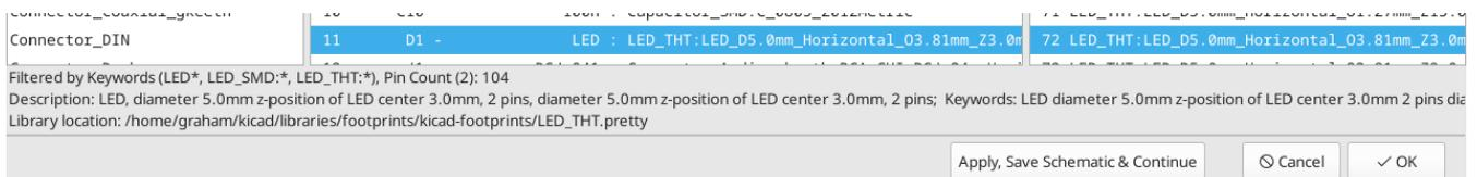
Multiple filters can be used at once to help narrow down the list of possibly appropriate footprints in the footprint pane. The symbols in KiCad's standard library define footprint filters that are designed to be used in combination with the pin count filter.
