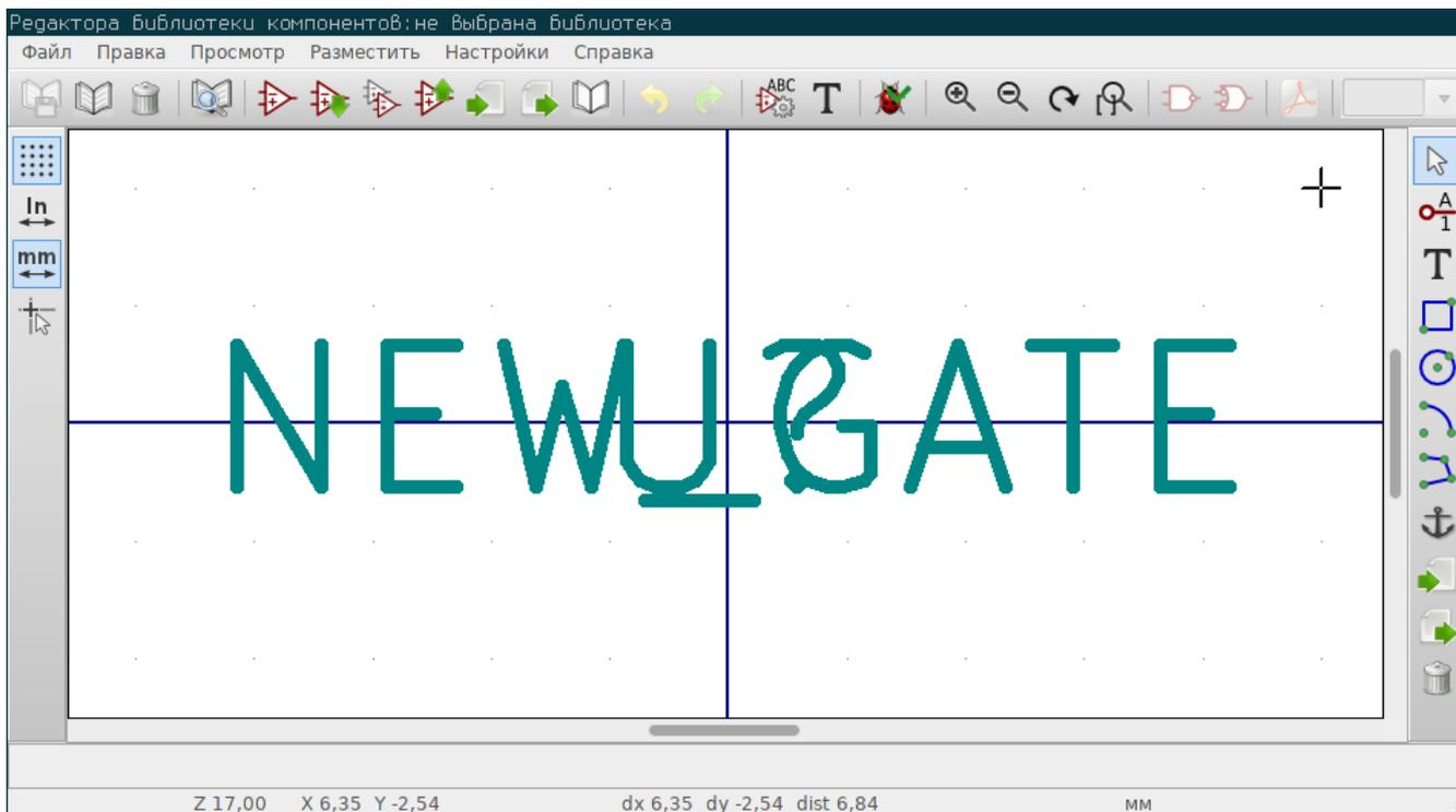
The blue cross in the center is the symbol anchor, which specifies the symbol origin i.e. the coordinates (0, 0). The anchor can be repositioned by selecting the
