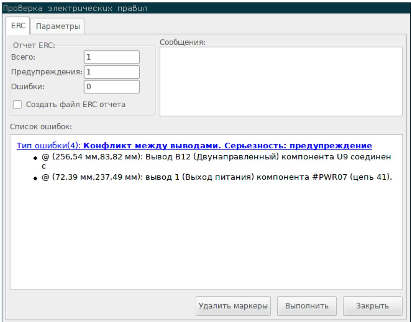
Any warnings or errors are reported in the **Violations** tab, and markers for each violation are placed in the schematic so that they point to the relevant part of the schematic. Warnings are indicated by yellow arrows, and errors have red arrows. Excluded violations are shown as green arrows.
